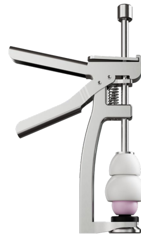
Figure 54. Maintain alignment of the liner to the axis of the support cone.
